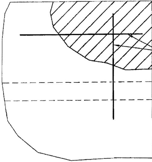
EPOXY IN (2) #4 DOWELS INTO DOUBLE TEE FLANGE, FORM UNDERSIDE OF SURFACE, PLACE BONDING AGENT ON EXISTING CONCRETE AND PLACE PRE-PACKAGED CONCRETE PATCH
