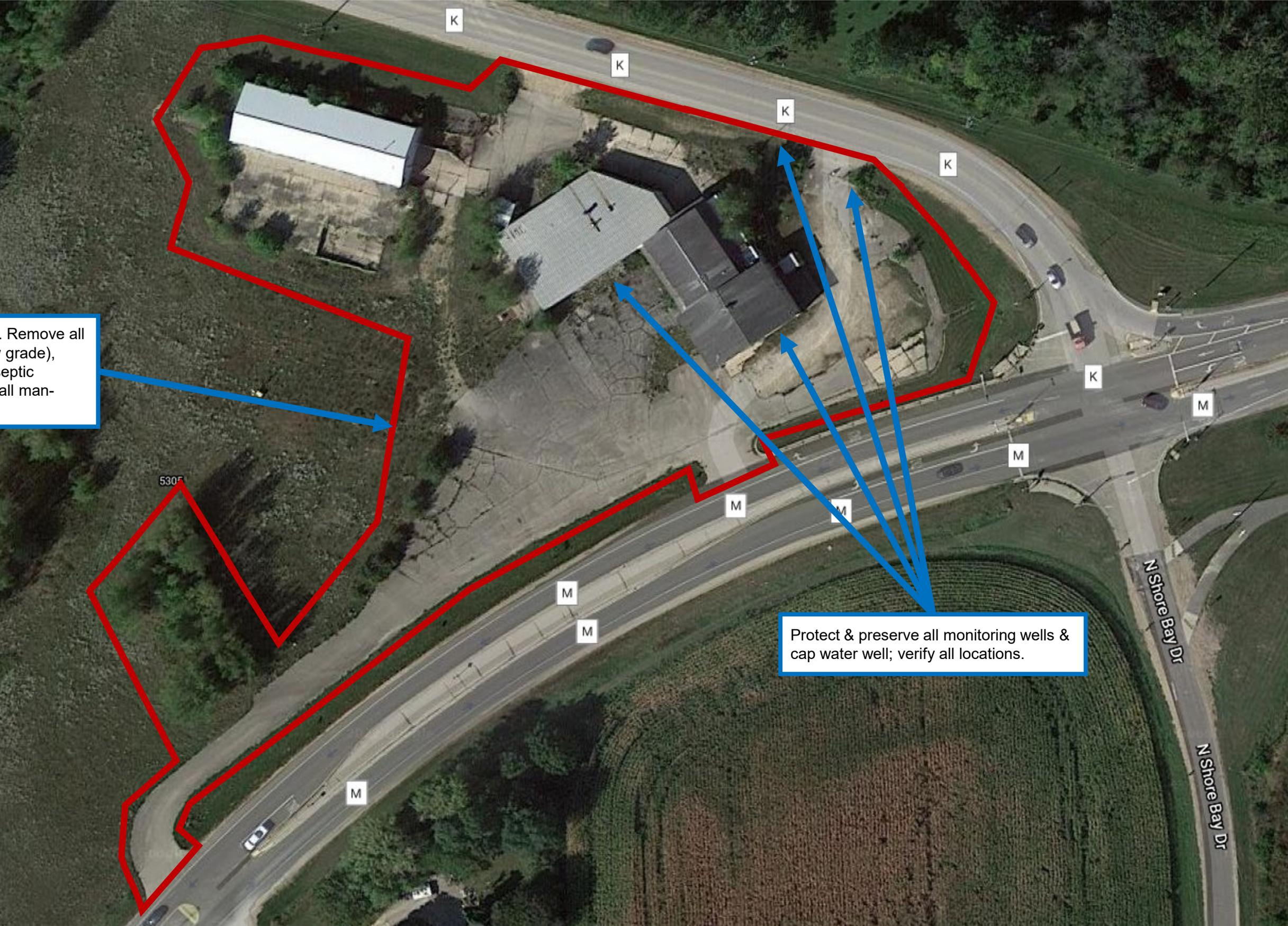
Limits of demolition work. Remove all buildings (above & below grade), vegetation, site utilities, septic system, hard surfaces & all man-made items
