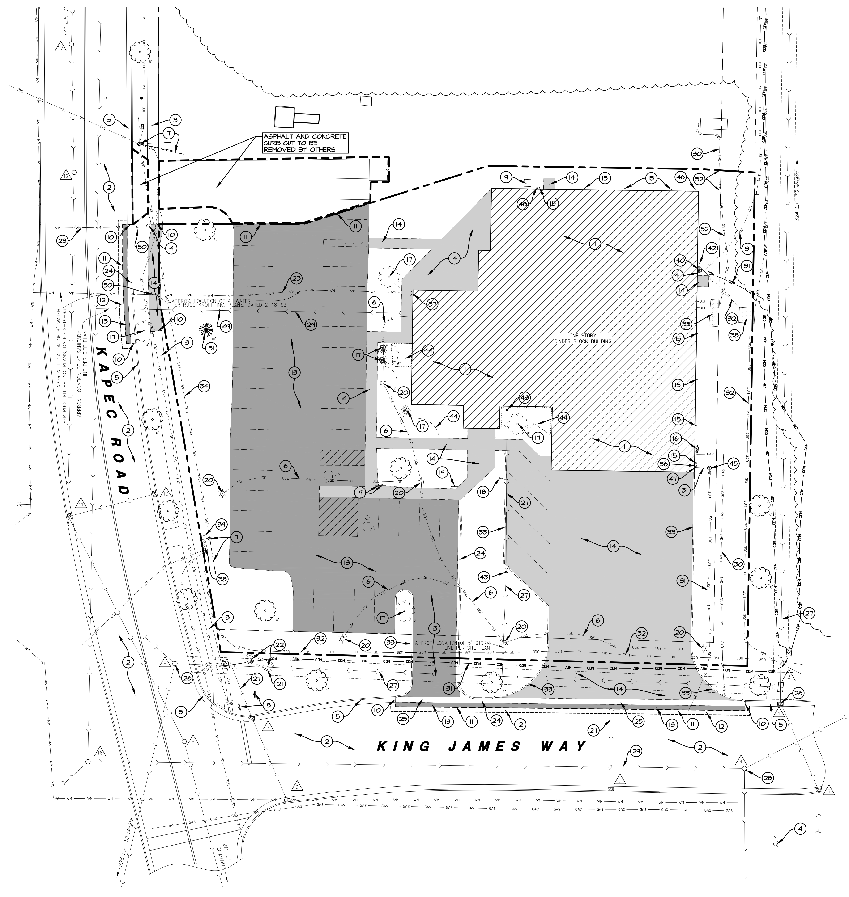
1 SITE DEMOLITION PLAN SCALE 1" = 20'
