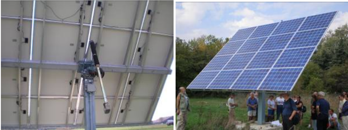
Figures 14 & 15 Back and front side of a dual-axis tracker, which follows the sun's apparent movement east to west and up and down daily.
