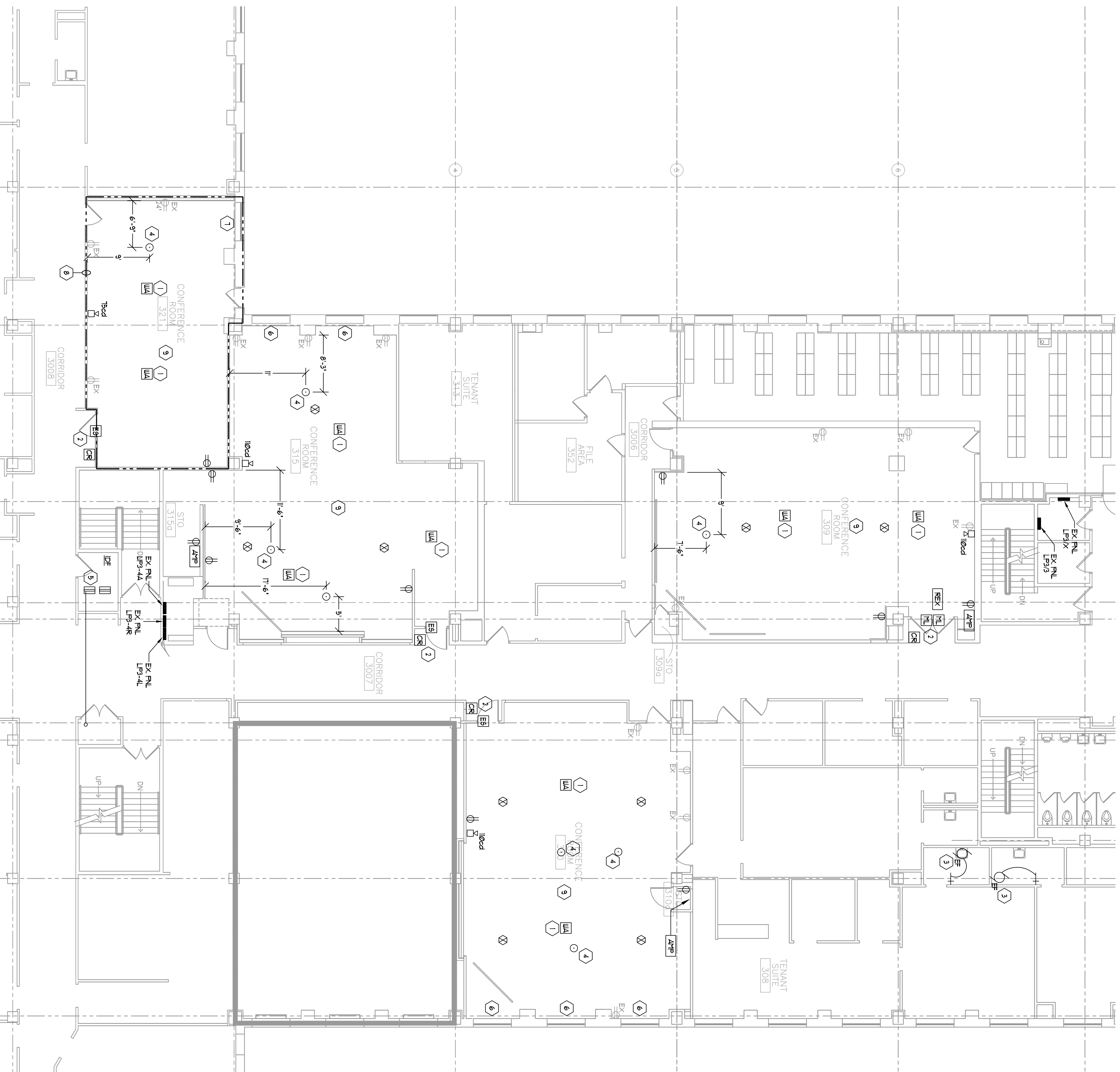
1 PARTIAL THIRD FLOOR POWER PLAN 1/8"=1'-0"
