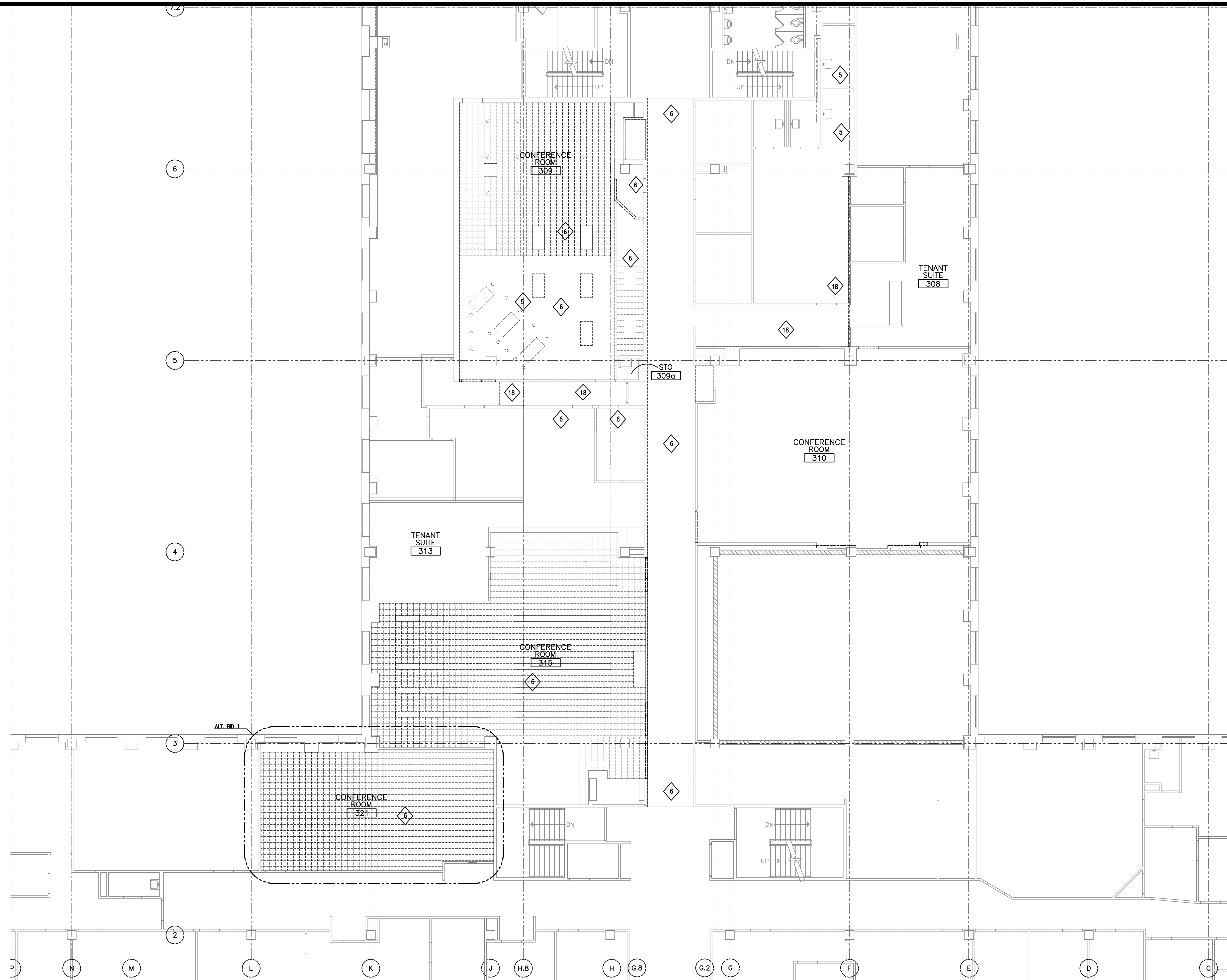
1 THIRD FLOOR AND REFLECTED CEILING DEMOLITION PLAN 1/8"=1'-0"
