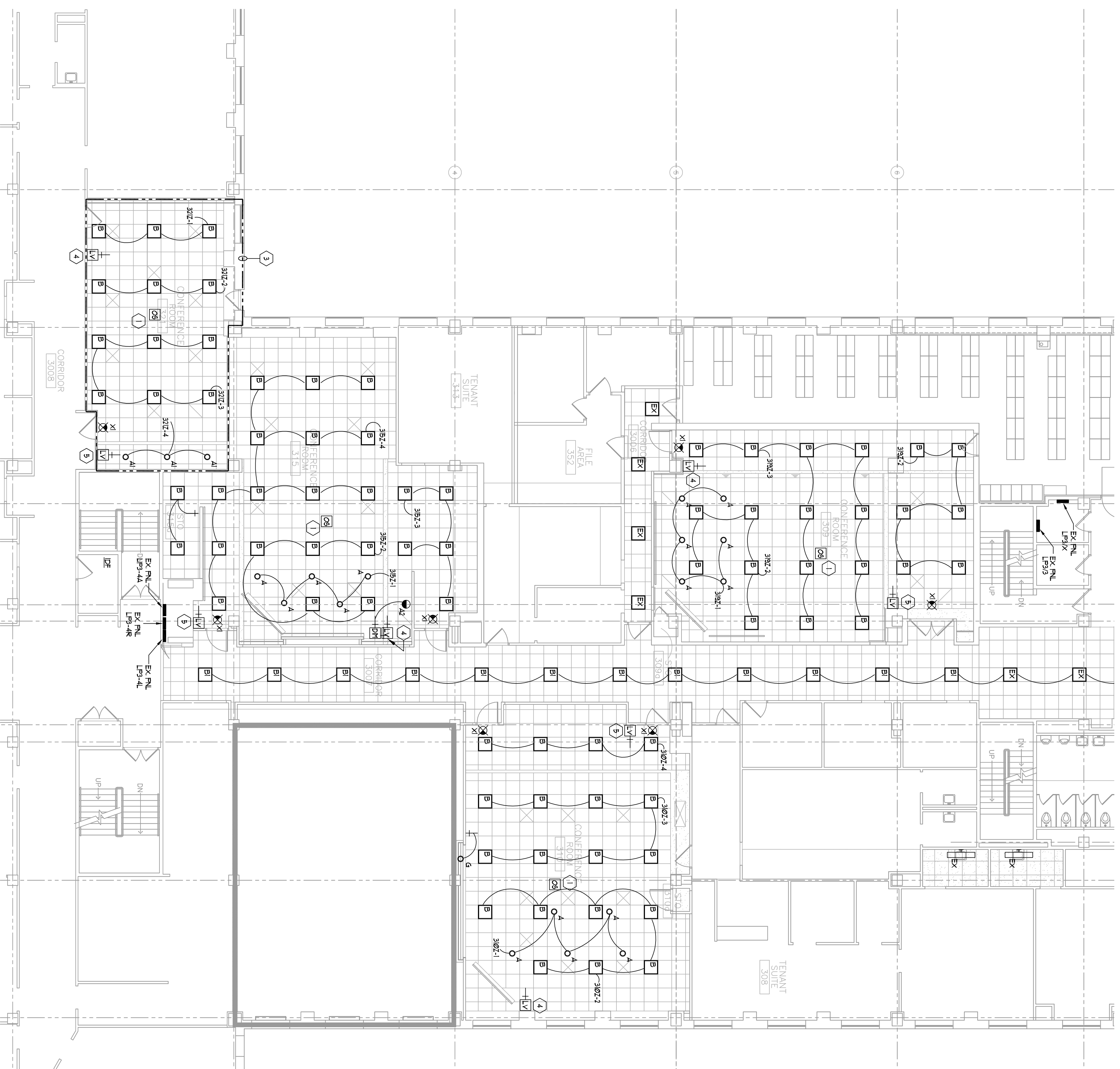
1 PARTIAL THIRD FLOOR LIGHTING PLAN 1/8"=1'-0"
