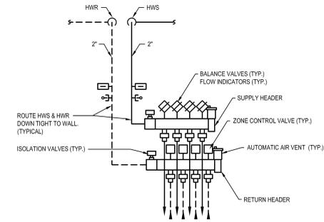
**2** RADIANT FLOOR HEATING MANIFOLD DETAIL
