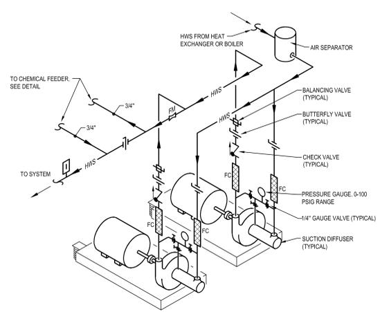
**7** DUPLEX BASE MOUNTED HOT WATER PUMP PIPING DETAIL
