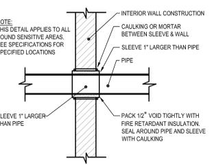
**6** PIPES THROUGH WALLS DETAIL
