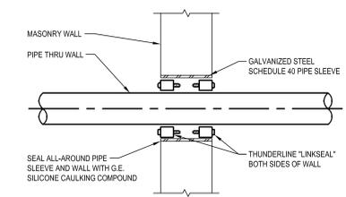
**3** PIPE THROUGH EXTERIOR BELOW GRADE WALL DETAIL
