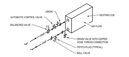
**9** TYPICAL PIPING TO HOT WATER BOOSTER COIL DETAIL
