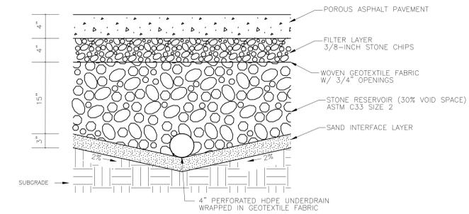
5 POROUS ASPHALT PAVEMENT SECTION
