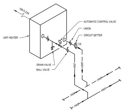
**10** HOT WATER UNIT HEATER PIPING DETAIL
