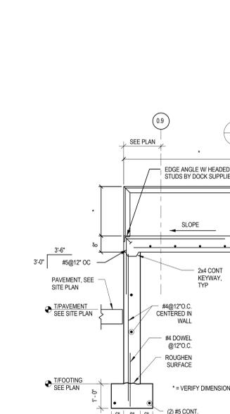
25 TYP. ISOLATION JOINT AT INTERIOR COLUMN
