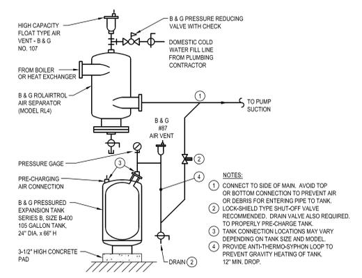
**2** VERTICAL EXPANSION TANK WITH AIR SEPARATOR DETAIL
