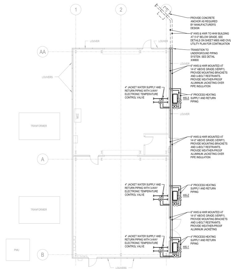
**1** FLOOR PLAN - HVAC PLAN
