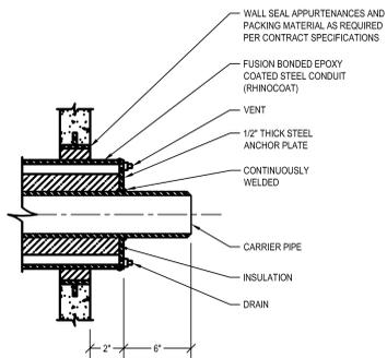
**10** CONDUIT END SEAL DETAIL
