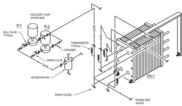
**5** PLATE AND FRAME TYPE HEAT EXCHANGER PIPING DETAIL
