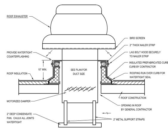
**8** TYPICAL ROOF EXHAUSTER DETAIL WITH CONDENSATE PAN
