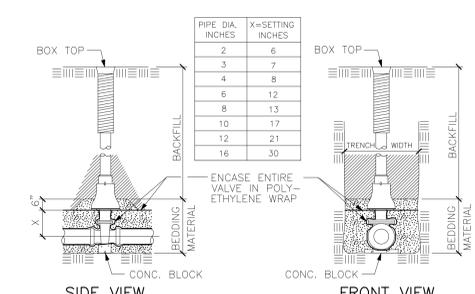
9 STANDARD GATE VALVE BOX SETTING DETAIL
