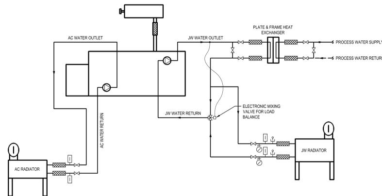
**4** JACKET WATER RECOVERY WITH TWO LOOP COOLING SCHEMATIC
