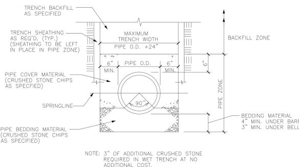
4 CLASS "C" BEDDING DETAIL FOR STORM SEWER
