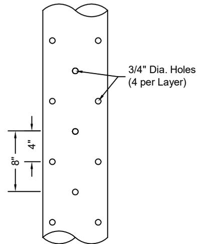
Drilled Pipe Section
