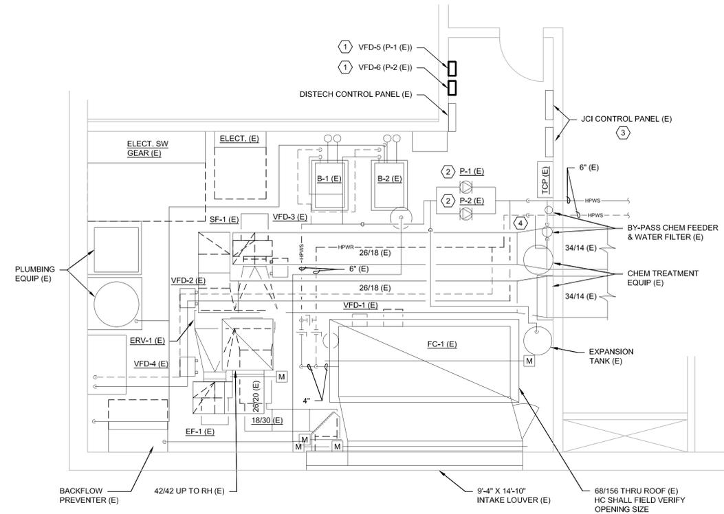
**2** MECHANICAL ROOM NEW WORK PLAN - HVAC
