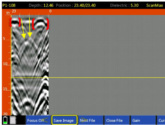
GPR data screenshot- relevant data screenshots of areas 1&2- Red brackets represent non grouted cells of CMU block and yellow arrows represent vertical bars marked during the time of the scan. (short scan)
