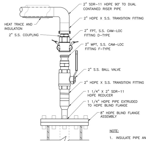
**WET WELL DISCHARGE PIPE ASSEMBLY**
