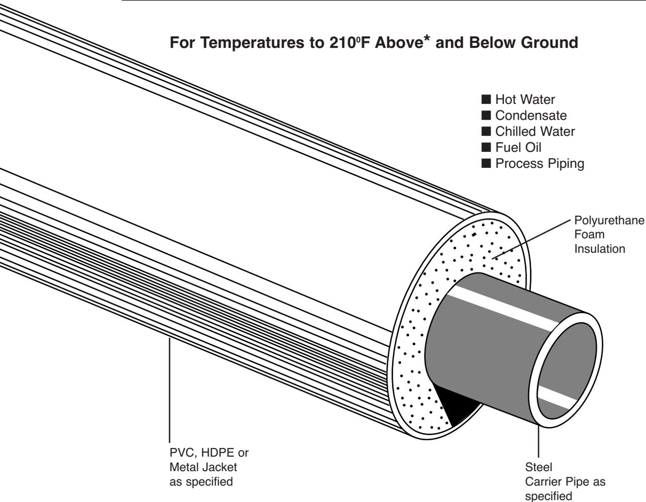
Rovanco's Steel System is designed for piping systems above or below ground suitable for inside or outside applications. High quality polyurethane foam insulation combined with a durable watertight jacket supplied in 20' or 40' random lengths, means an economical, high-quality system.
