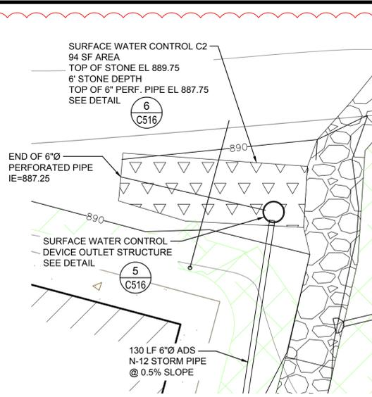
**SURFACE WATER CONTROL DEVICE OUTLET STRUCTURE ELEVATIONS**
