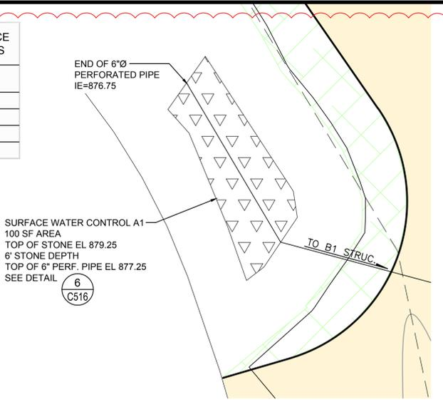
**SURFACE WATER CONTROL DEVICE A1**
