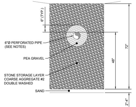
**SURFACE WATER CONTROL DEVICE TYPICAL SECTION**
