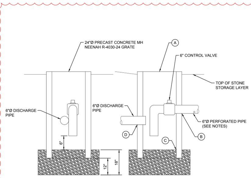
**SURFACE WATER CONTROL DEVICE OUTLET STRUCTURE**
